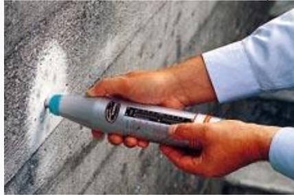
Original Schmidt Concrete Test Hammer
